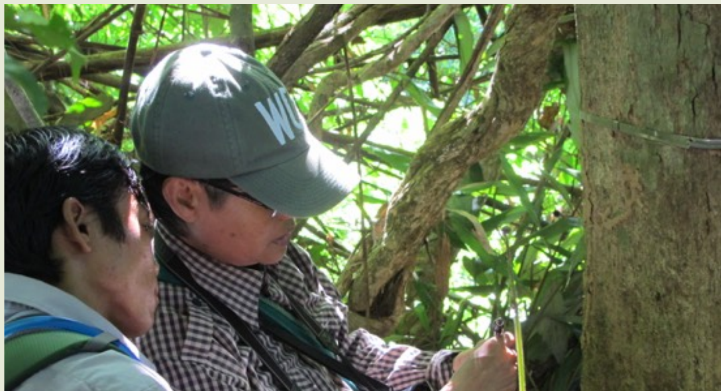
Daw Myint Myint Oo (WCS) and U Linn Zaw (Nam Sabi) carefully review the caliper before recording the diameter increment of the kyauk ta mar tree outside of Nam Sabi that was fitted with a dendrometer band (shown upper right). [NOTE: The tree had grown 0.37 cm in diameter in the five months since the band was placed around the tree].
