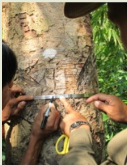
Making a growth band to fit around a Thin bone ( Alstonia rostrata ) tree.
